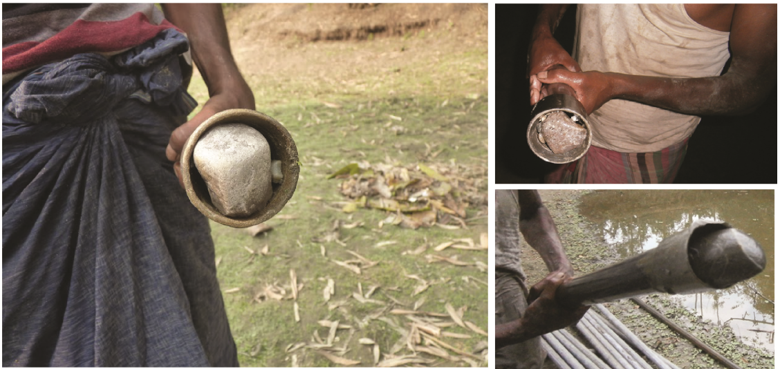
Figure 2.8: Images of pebbles and cobbles lodged in the drilling shoe.
