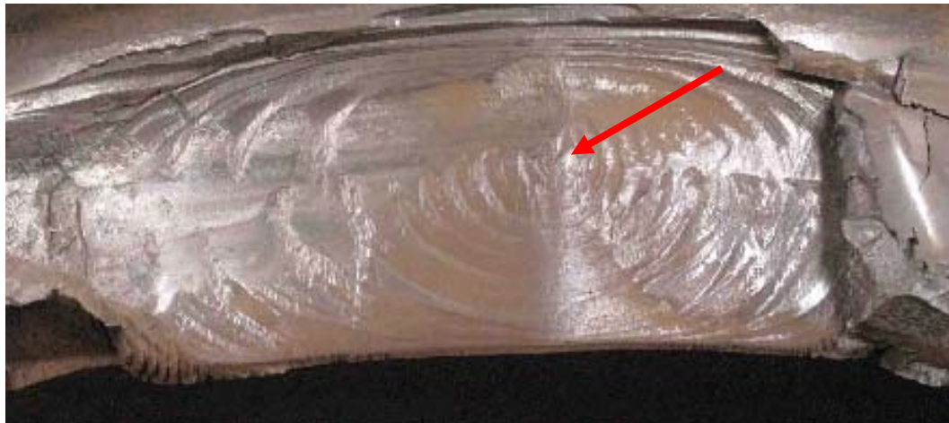
Figure 5. Photograph of wheel section showing the “bulls-eye” pattern of a shattered rim; arrow points to origin
