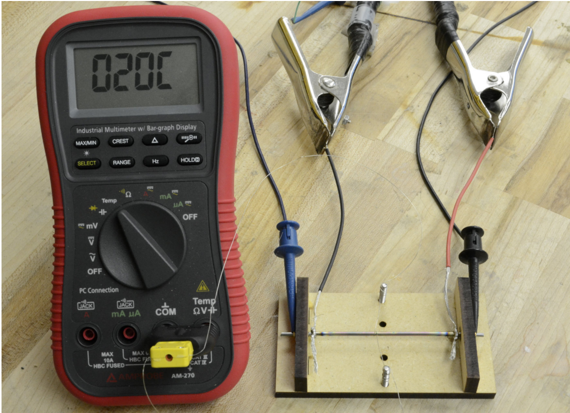
Figure 2.12: The experimental setup for collecting temperature data.
