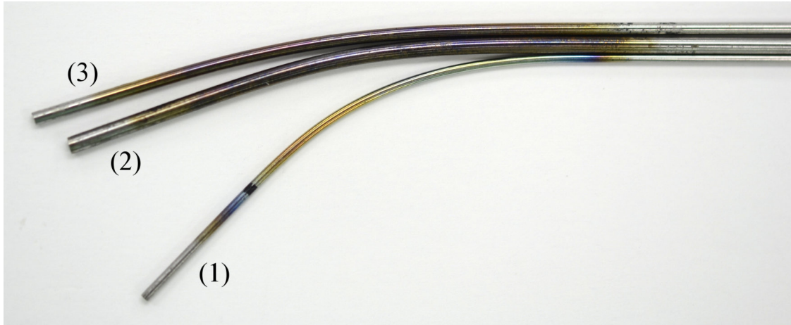
Figure 2.14: Multiple Nitinol tubes of varying diameters that have been shape set to different curvatures. This photograph was taken immediately after shape setting of each tube, before any additional cleaning or trimming operations. The coloration of the tubes in the heated region is a result of surface oxidation and fixture charring.
