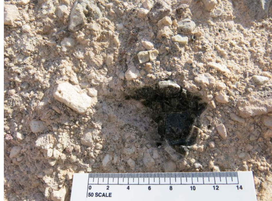
Perlitic black obsidian. Chemically identical to the pumice glass (phase assemblage is the same as well)
