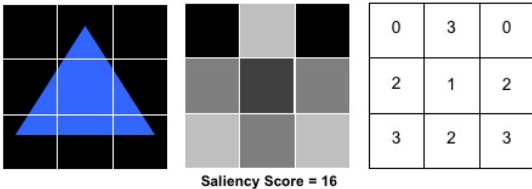
Figure 3.2 Sample calculation of saliency scores. A simplified depiction of how saliency scores were derived. The first panel represents the image. The second panel represents the saliency map for the image. The third panel is the numerical matrix of saliency values that the Saliency Toolbox uses to generate the saliency map, and the saliency scores were generated by summing the cells of the numerical matrix for the image, giving a saliency score of 16 for this example.
