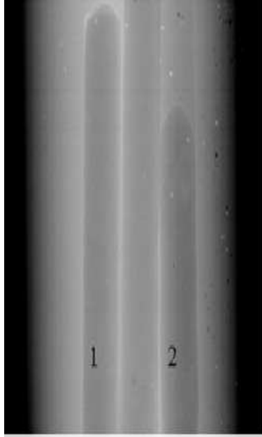
Figure 3.10: The phase-contrast radiographic image showing the two selected holes used in calculating the relative differences for this image.
