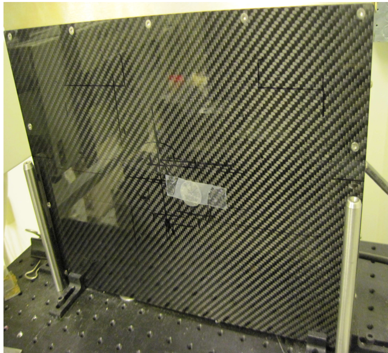
Figure B.1: SMAM II Mammography Detector. Note: A lead beam stop is attached to the detector.
