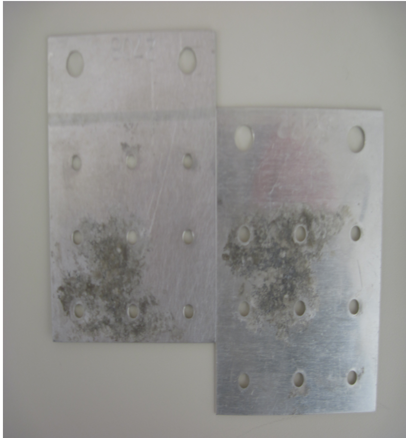
Figure 4.2: Disassembled aluminum lap joint with naturally formed corrosion provided by Wyle.
