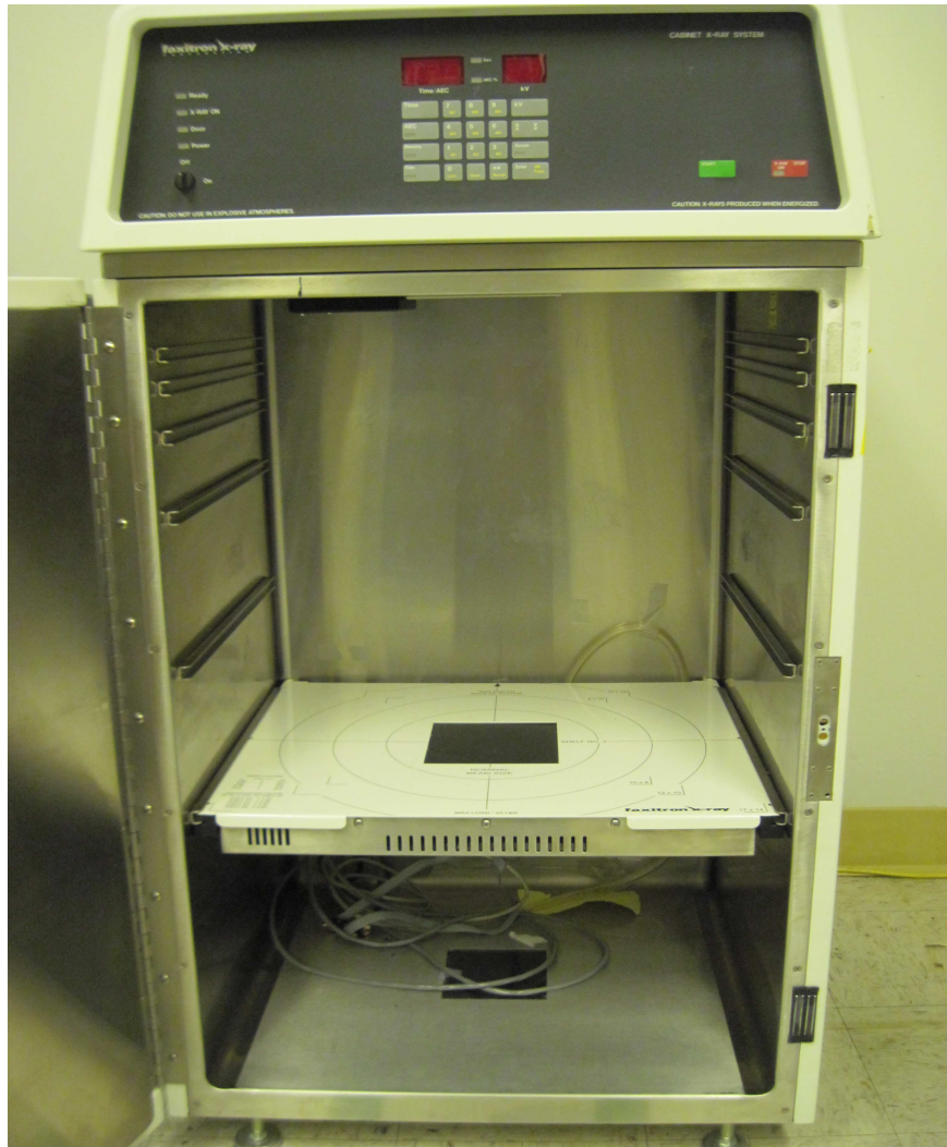
Figure B.4: Faxitron LX-60 with x-ray detector at shelf position 1.5.
