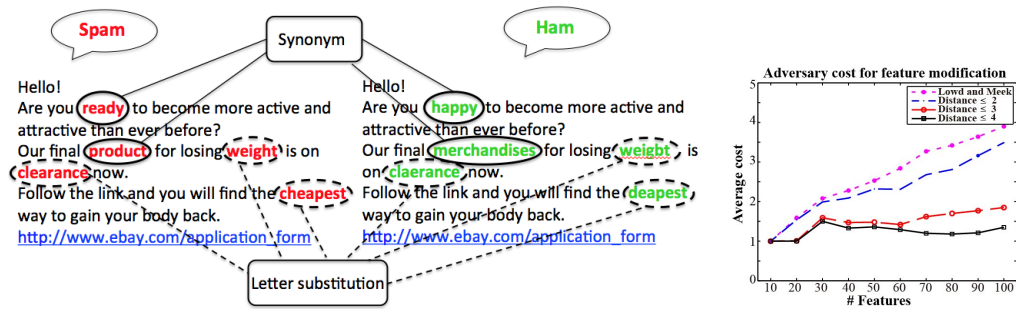
Figure 3.2: Left: illustration of feature substitution attacks. Right: comparison between distance-based and equivalence-based cost functions.
