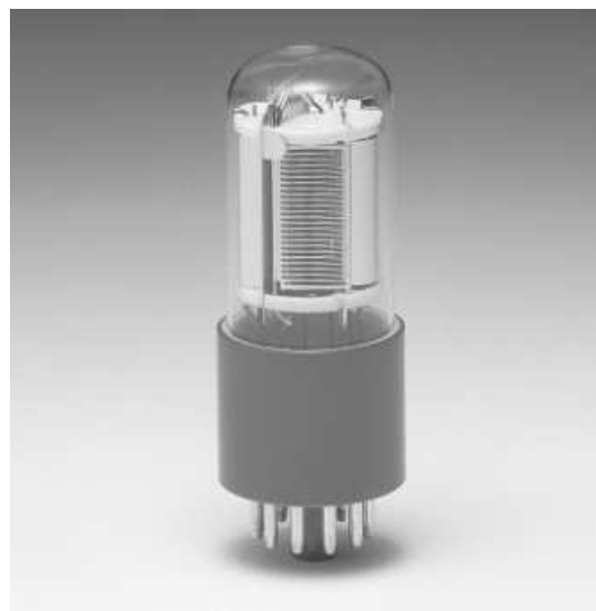
Figure 3.2: A picture of R4632 side-on PMT. From 'hamamatsu.com'
