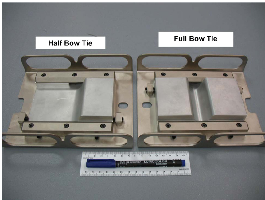
Figure II.3: Half and full bowtie filters placed in front of the x-ray source for kV-CBCT acquisition. (Reproduced from [32] with permission)
