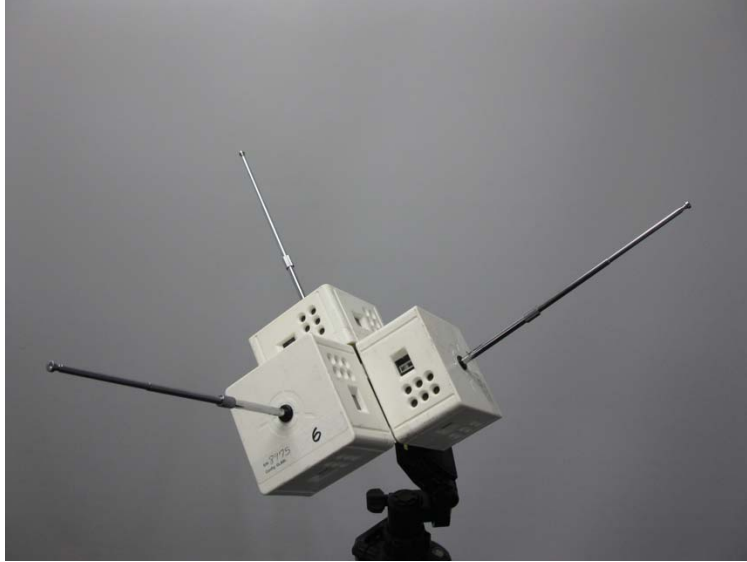
Figure 37: TripLoc antenna array implementation using three XSM motes. The name TripLoc comes from the fact that a triplet of nodes constitute an anchor node array in our localization scheme.
