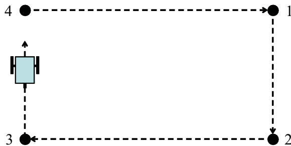
Figure 55: Waypoint Navigation. A mobile entity traverses the sensing region by navigating between position coordinates.
