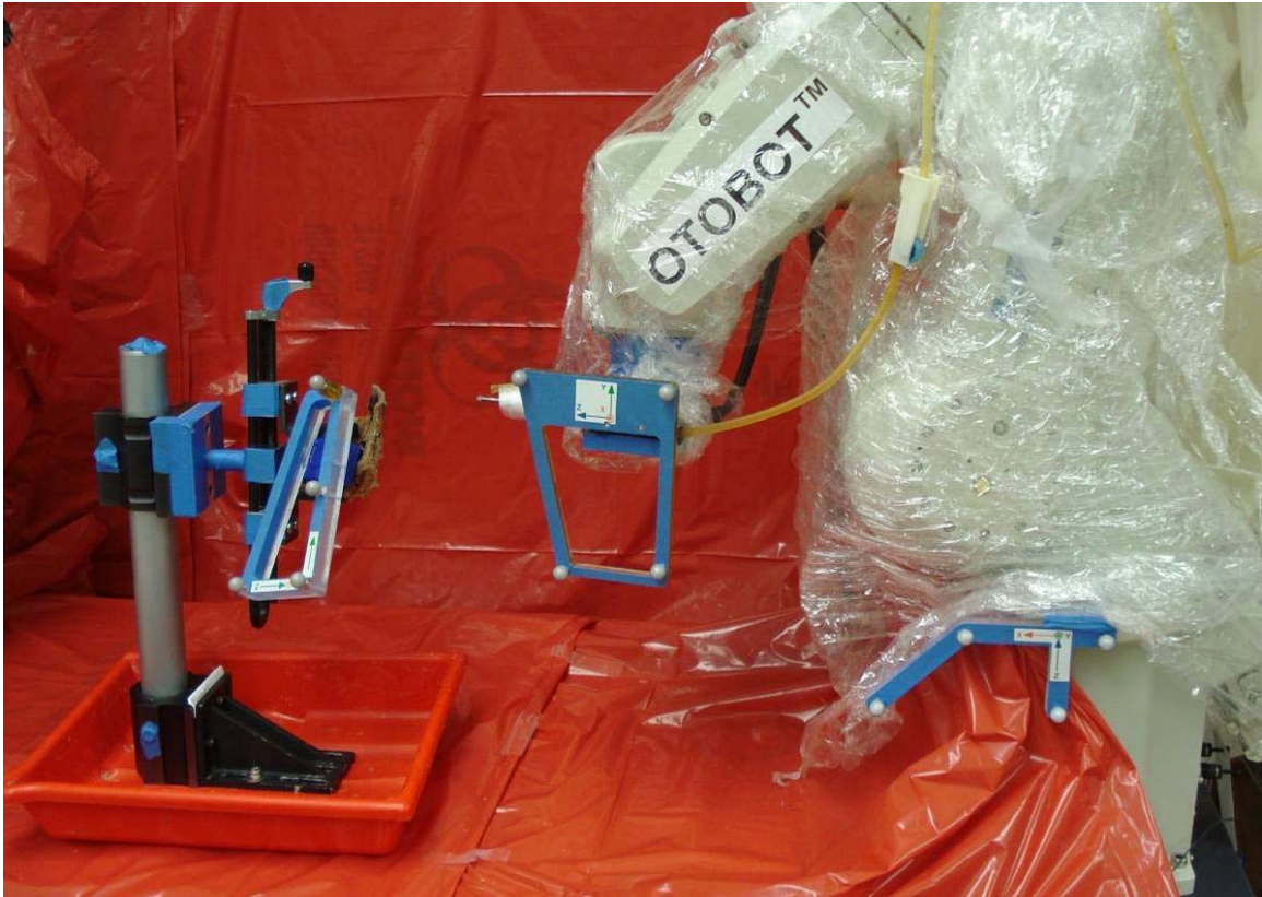
Figure 1. OTOBOT™ robotic system set up to perform mastoidectomy on patient (temporal bone specimen in this current study). The robotic system consists of a Mitsubishi RV-3S industrial robot controlled by custom software. Coordinate reference frames with markers are attached rigidly to the robot end effector, robot base, and patient to allow tracking of the movements of the robot, drill, and patient during milling. An NDI Polaris optical tracking system (not shown here) is used to track the markers.
