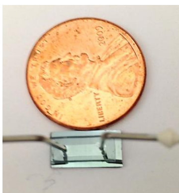
Fig. 30 Final microfluidic system with metal pin connection
