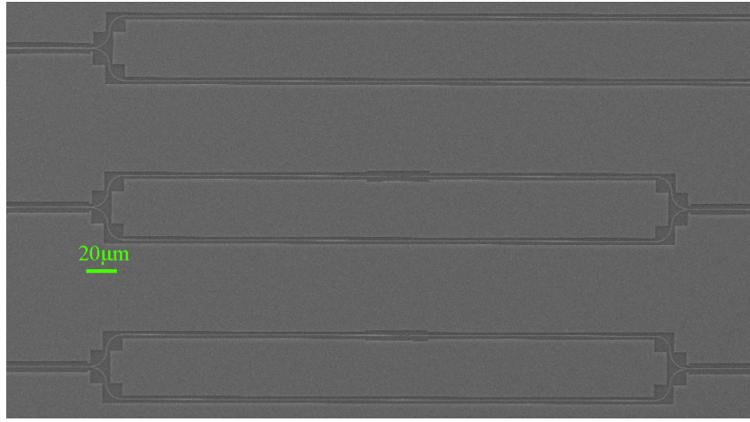
Fig. 3 SEM image of SOI based MZI
