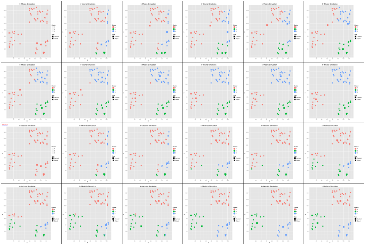
Figure 2: Comparison of k -Means and k -Medoids on identical data and initial centroids. Following different paths, each correctly identifies the three natural clusters. Note how the means glide between clusters, while medoids make distinct jumps.
