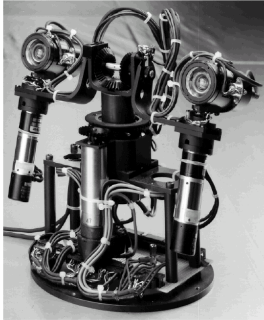
Figure 28: ESCHeR: ETL stereo head for robot vision [67]
