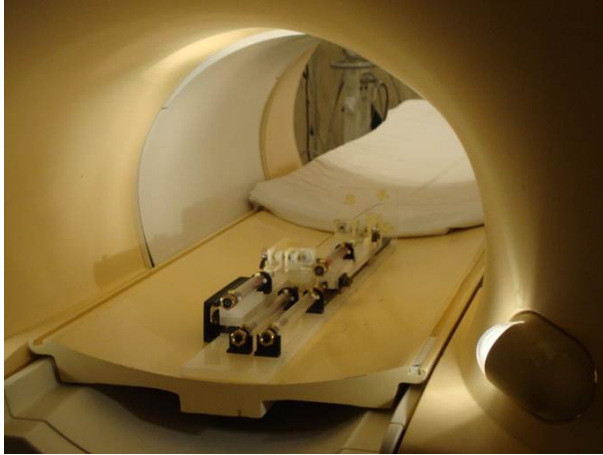
Figure 6.5: MRI-compatible robot in the 3T Philips Achieva scanner.
