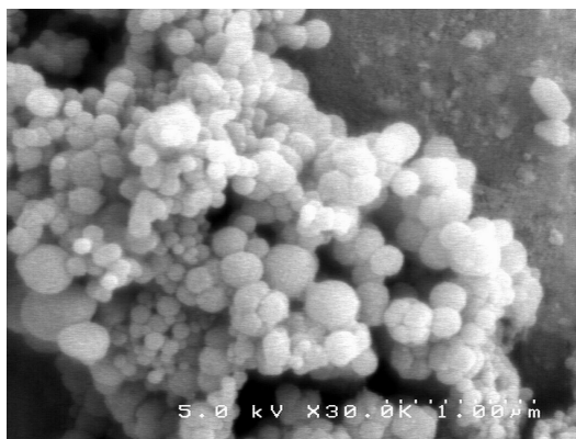
Figure 63. (Top) Visual confirmation of GO encapsulation. (Left) 6 mg/mL GO solution used in silica synthesis. (Center) Silica prepared and washed in water showing encapsulated GO. (Right) Silica prepared in the presence of GO and 0.1M phosphate buffer. (Bottom) SEM image of silica particles formed in water and containing GO.
