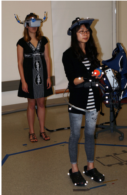
Figure 3.10: A participant acting as an observer in the experiment. The assistant is wearing the 6 tracking objects on her feet, hands, waist, and head so that a character can be created for the participant to view in the VE.
