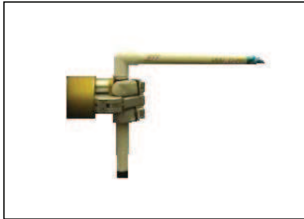
Figure 9: Example of an industrial manipulator holding a truss pipe.
