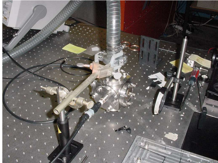
Figure 10. A photograph of the setup. The front window of the mini-chamber faces the optical lens where the laser passes through. The lens controls the focal point of the laser.
