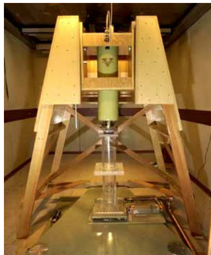
Figure 4.6: Photograph of the entire system including the non-magnetic scanning stage and SQUID Dewar wooden support structure. The SQUID microscope system is housed inside a 3 layer \mu -metal magnetically shielded room.
