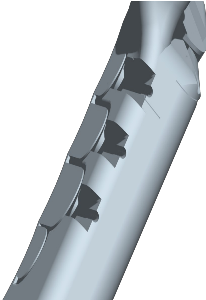
Figure 12. Joystick finger load cell enclosure
