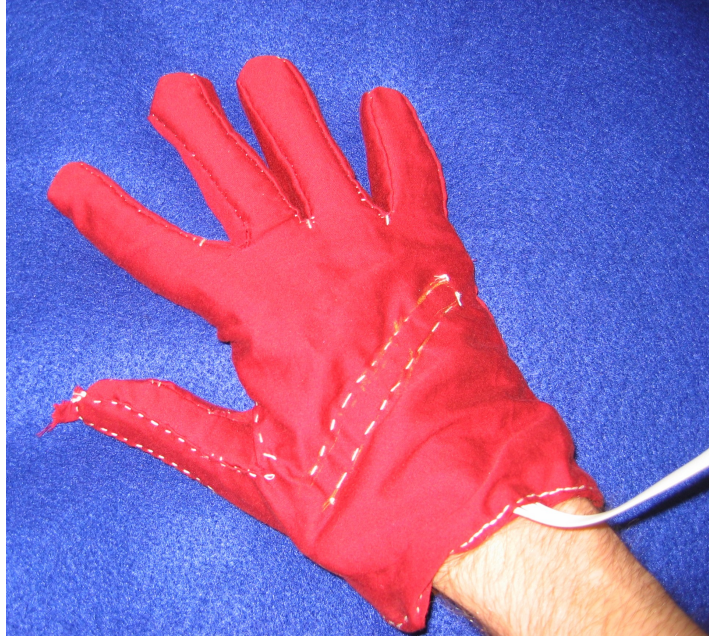
Figure 6. Preliminary position-based finger sensor package
