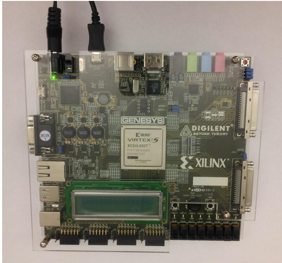
Fig. VI-33 Xilinx Virtex-5 FPGA used to implement the ECC and the fault injection block. The FPGA is mounted on a GENESYS Diligent development board.
