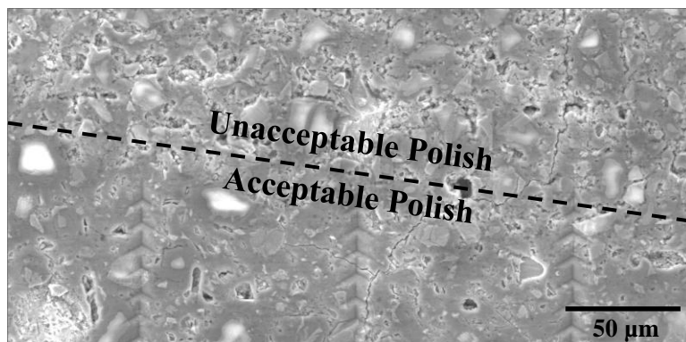
Figure 4.2. SEM image showing areas of a cement-based composite considered to have an acceptable and unacceptable polish for nanoindentation.
