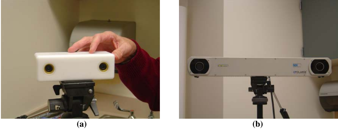
Figure 20. Tracking systems. (a) MicronTracker, (b) Hybrid Polaris.
