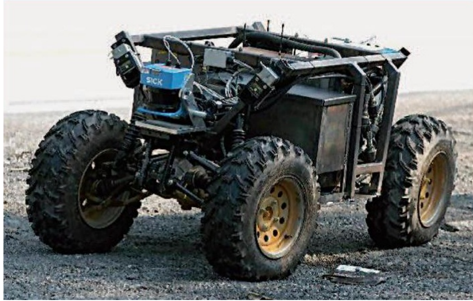
Figure II.2: The Groundhog, CMU's autonomous mine mapping robot.
