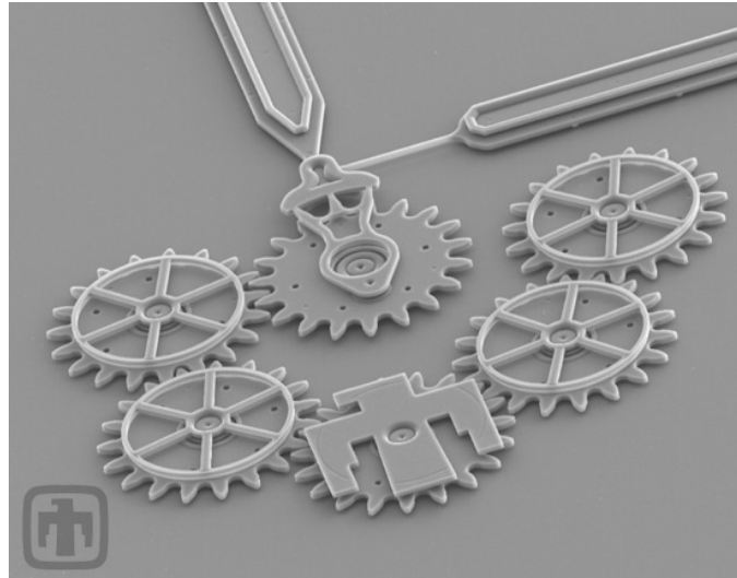
Figure 2.1. Scanning electron micrograph from Sandia National Laboratory demonstrating intricate fabrication capabilities for MEMS components. Image courtesy of Sandia National Laboratories, SUMMiT(TM) Technologies, http://www.mems.sandia.gov .
