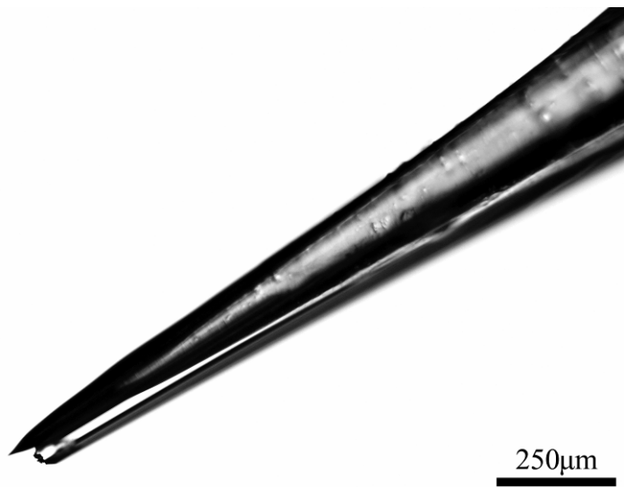
Figure 5-2. Photomicrograph of the tip if the injectrode, custom made in our lab. See text for the details of making this injectrode.
