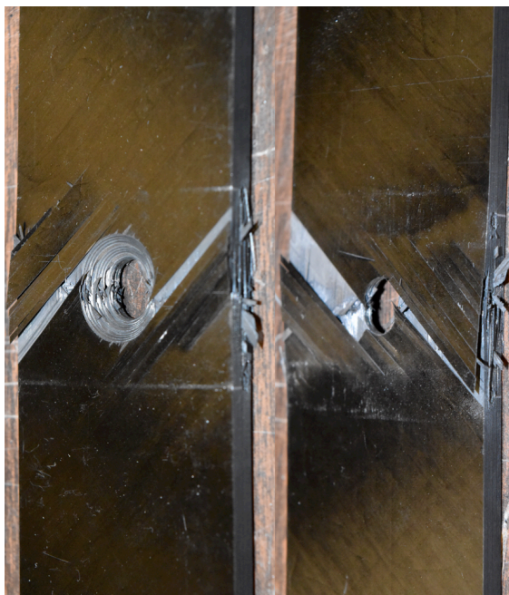
Figure 27. Open Hole experimental overall damage patterns for qualitative comparison
