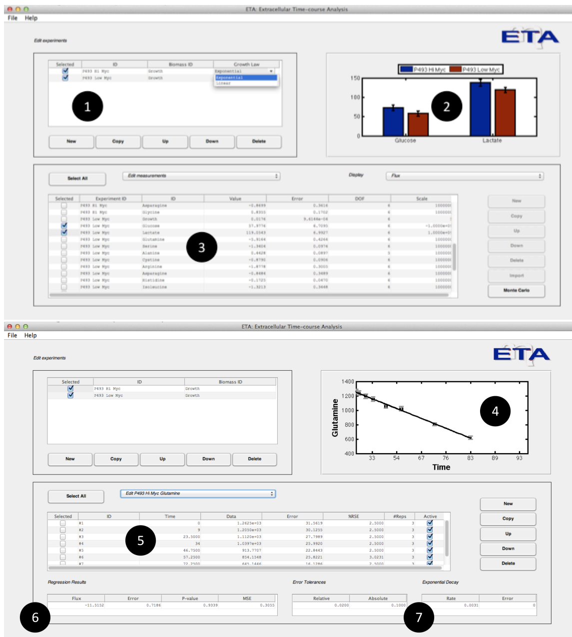
Figure 3.3 Features of the ETA Software Package. (A) Users are able to (1) create new experimental time courses and view the calculated rate (or yield) estimates and associated uncertainties in both (2) graphical and (3) tabular formats for either exponential or linear growth models. (B) When a single measurement is selected, the program allows the user to (4) graphically assess the goodness-of-fit, (5) enter and select raw data for regression, and (6) view the calculated rates along with the p-value and mean-square error of the fit. Adjustable error tolerances and first-order degradation parameters can also be supplied by the user (7).
