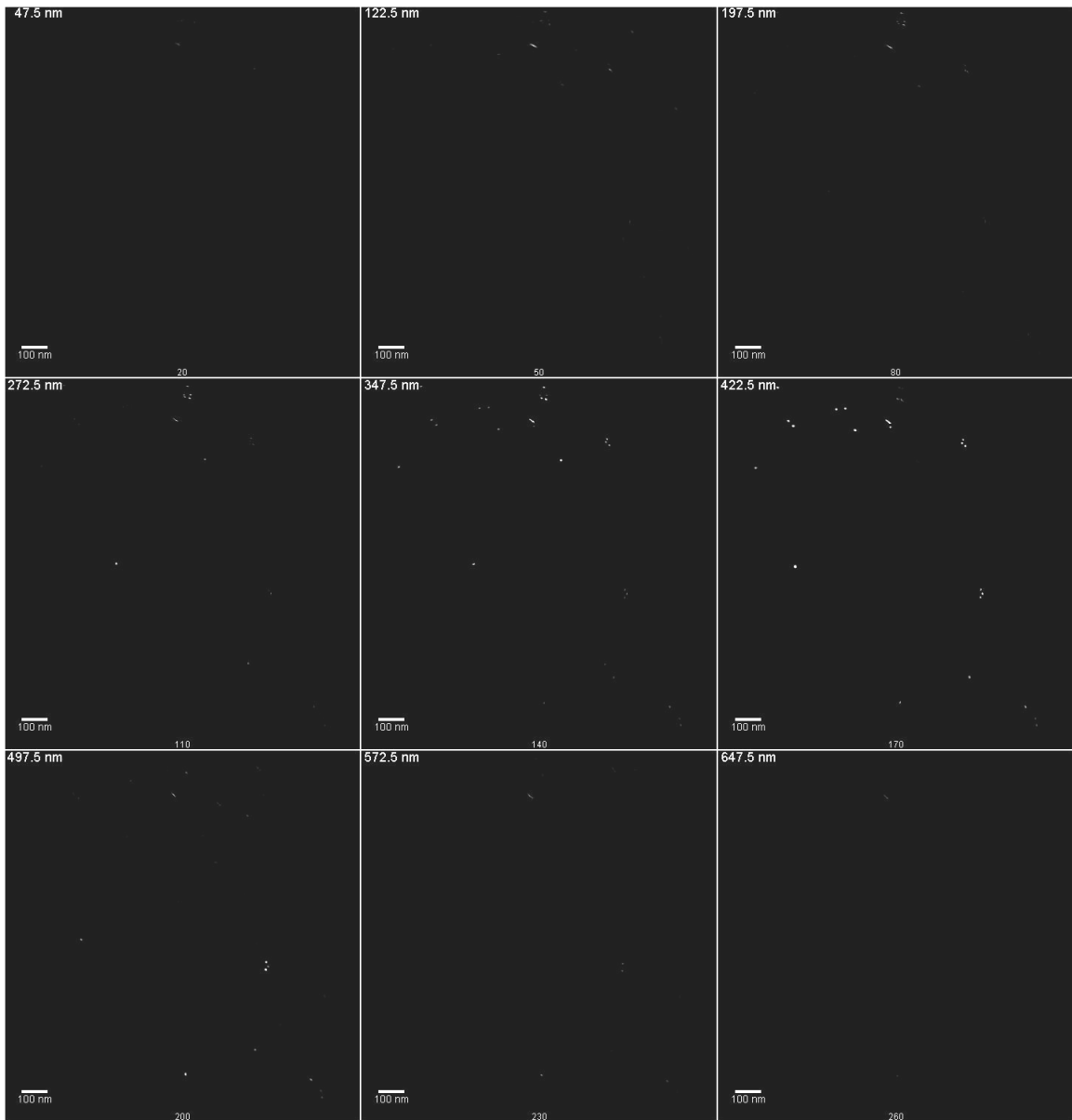
Figure 29: The same image frames, as shown in Figure 27, after deconvolution. The image contrast and brightness have been adjusted to highlight the positions of the gold nanoparticles. The majority of the particles are in frame 170. The deconvolved images contain less noise than the non-deconvolved images.
