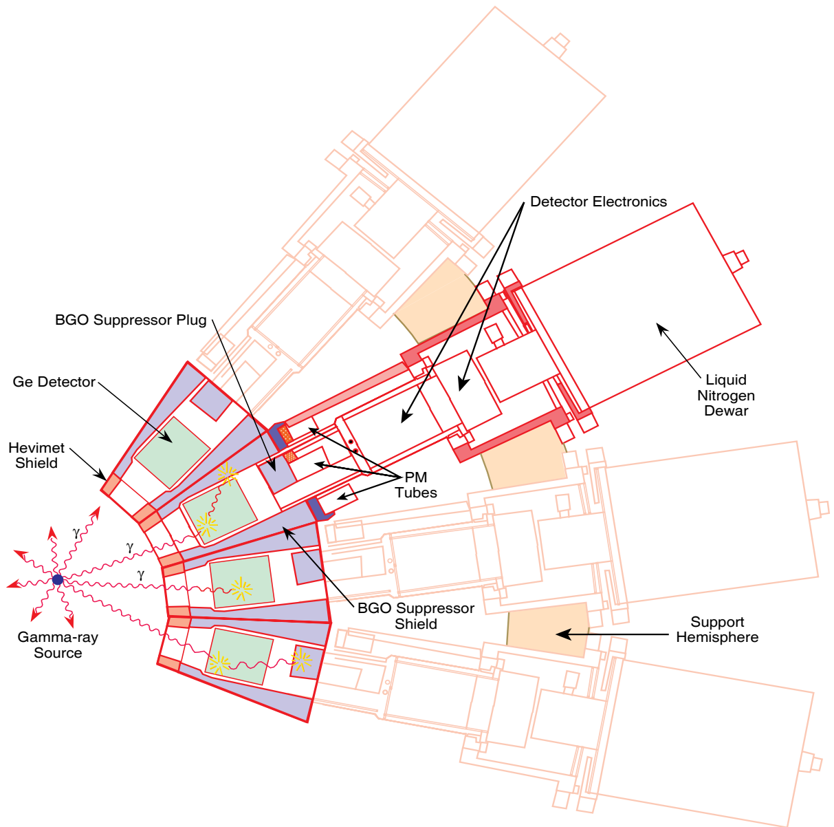
Figure 12: Gammasphere cross-section schematic [GAM]
