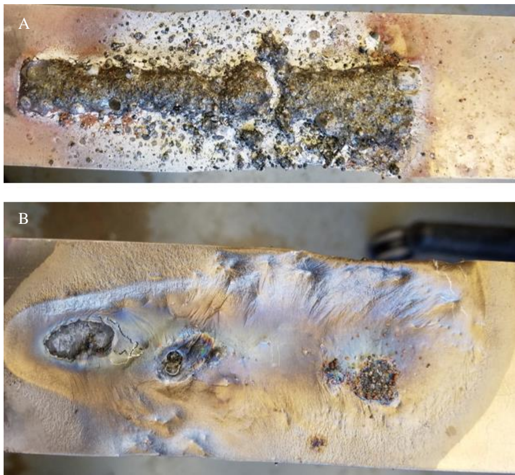
Figure 20 –A) Top side of ignition 3. B) Bottom side of ignition, showing small holes
