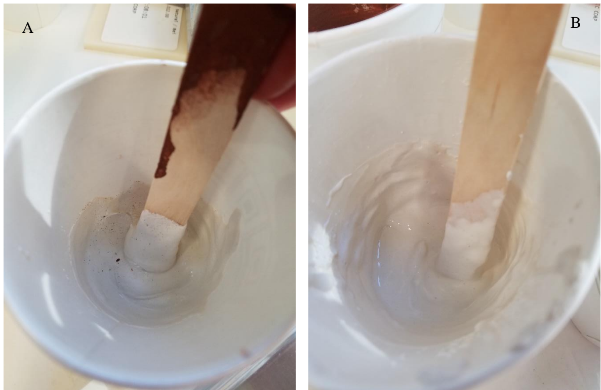
Figure 12 – A) Plaster without tartaric acid and B) Plaster with tartaric acid
