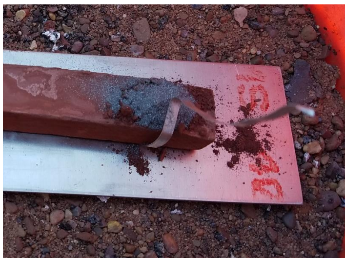
Figure 17 – Thermite Ignition Setup
