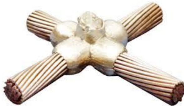
Figure 4 –Thermite Weld of Copper Cables [6]
