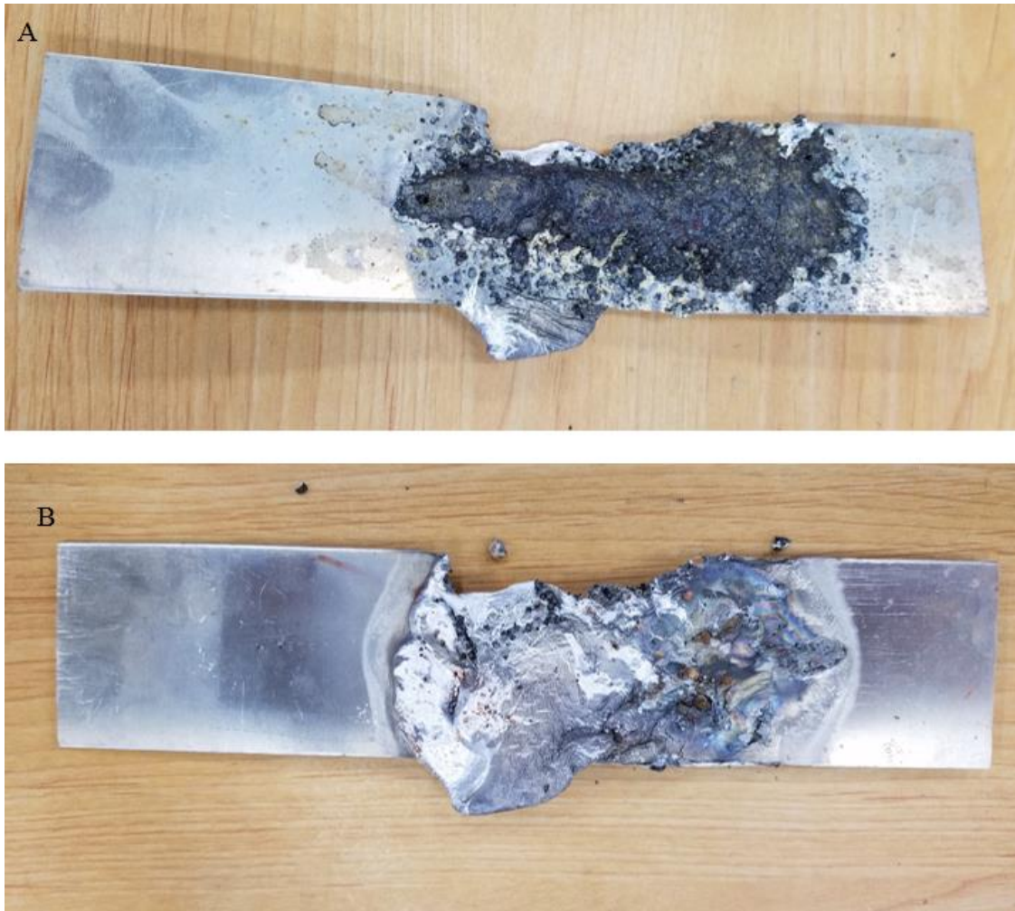
Figure 18 – A) Top side of ignition and slag. B) – Back side of ignition, with notable deformation
