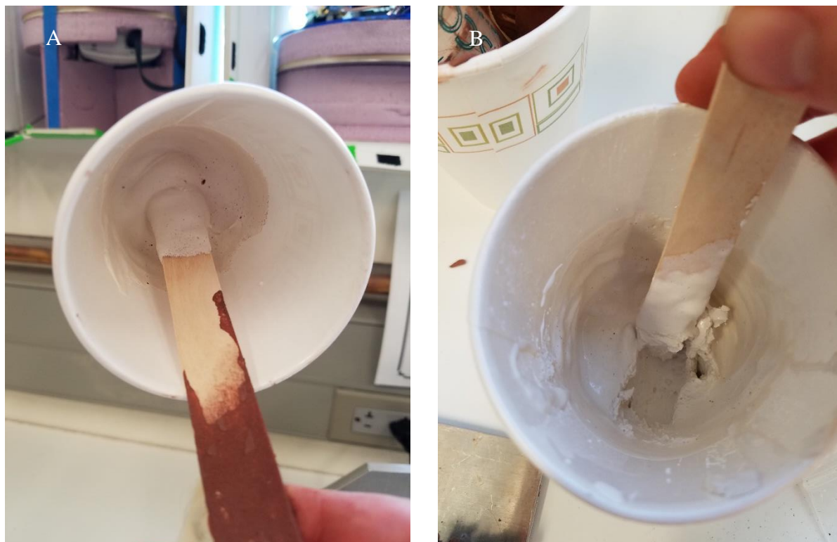
Figure 13 – A) Sample without tartaric acid, suspended upside down. B) Sample with tartaric acid, still in workable stage
