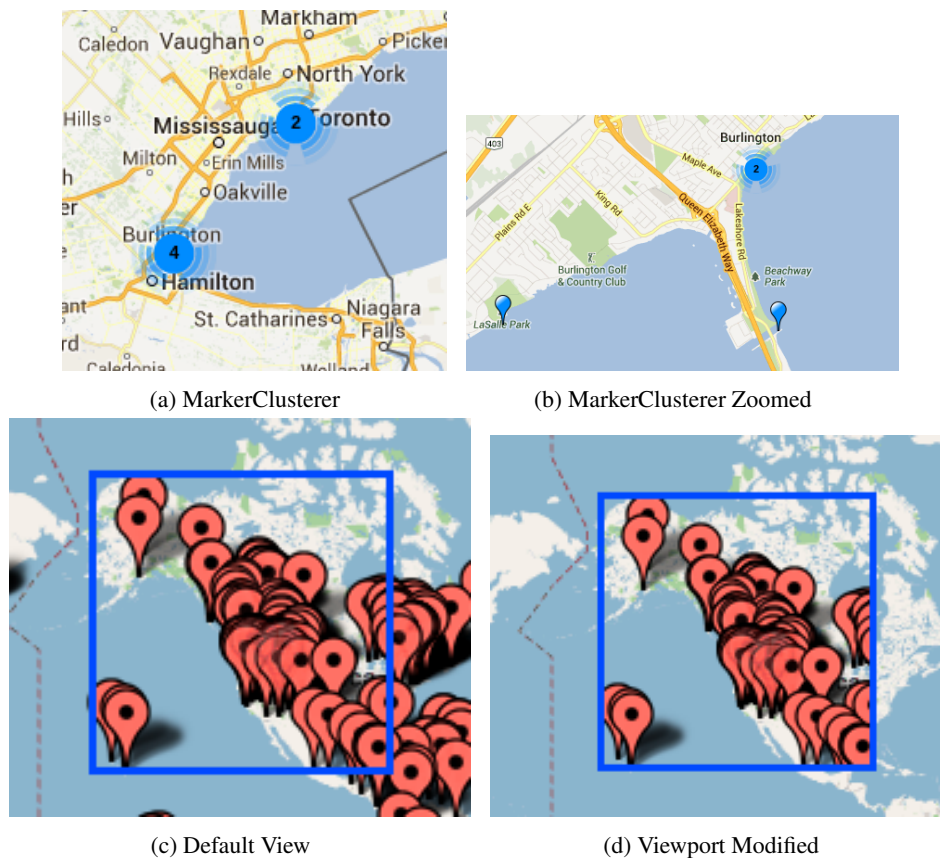
Figure II.5: A Markerclusterer (2009) visualization for Burlington shown in a default view (a) and a zoomed in view (b). Zooming in breaks contained POIs into smaller clusters or individual POIs. Zooming also effects visualized information in viewport management techniques (c) and (d).
