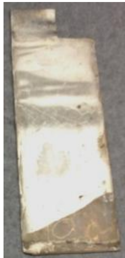
Figure 3.4 - Silver plate. The silver plate serves as a conduction path for the current to flow through to the Si which serves as the anode during the electrochemical etch.
