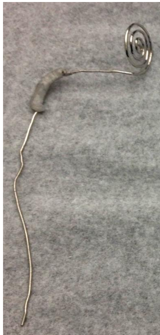
Figure 3.2 - Platinum wire. The platinum serves as the cathode when electrical current is passed during etching.
