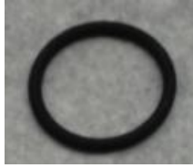
Figure 3.3 - O-ring. 2 cm 2 in area, the O-ring serves as a seal and is placed between the Si substrate below and the etch cell above.
