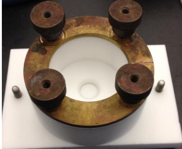
Figure 3.1 - Teflon etch cell. The etch cell contained a hole of 2 \text{ cm}^2 area in the bottom which demarcates the area to be etched in the Si substrate place below
