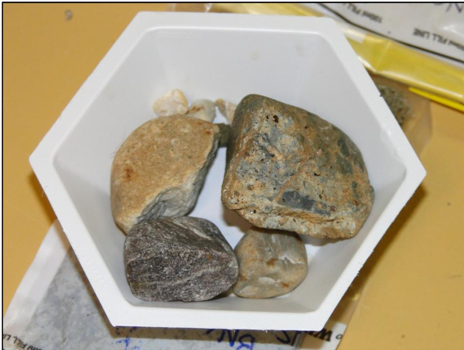
**Figure 20. The abundance of fractured clasts is attributed the drilling method. This is important to consider when analysing the dry sieve results of gravel clast sizes and abundances.**
