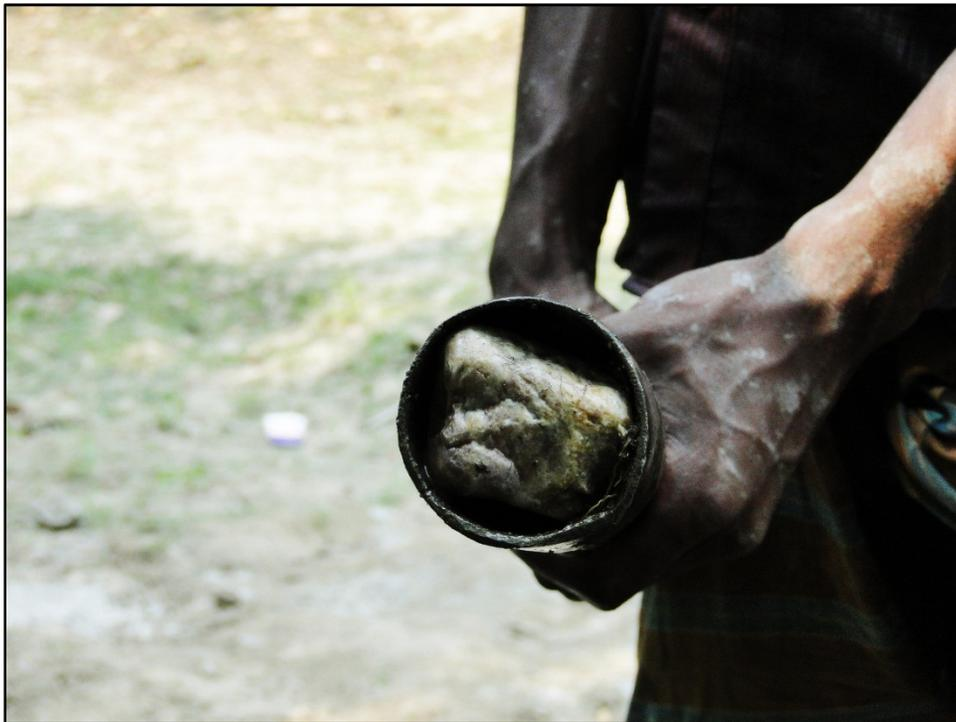
**Figure 18. A gravel clast lodged in the 2 inch diameter drill string.**
