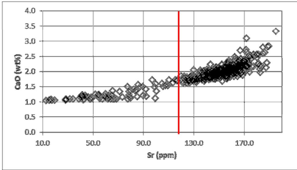
**Figure 12. A positive correlation between CaO (wt%) and Sr (ppm) reveal that an increased presence of Ca-bearing minerals is a major control on Sr (ppm) in matrix sediments. Note that all of the >120 ppm population show CaO > 1.5 wt%. The red line marks 120 ppm. (n=443)**
