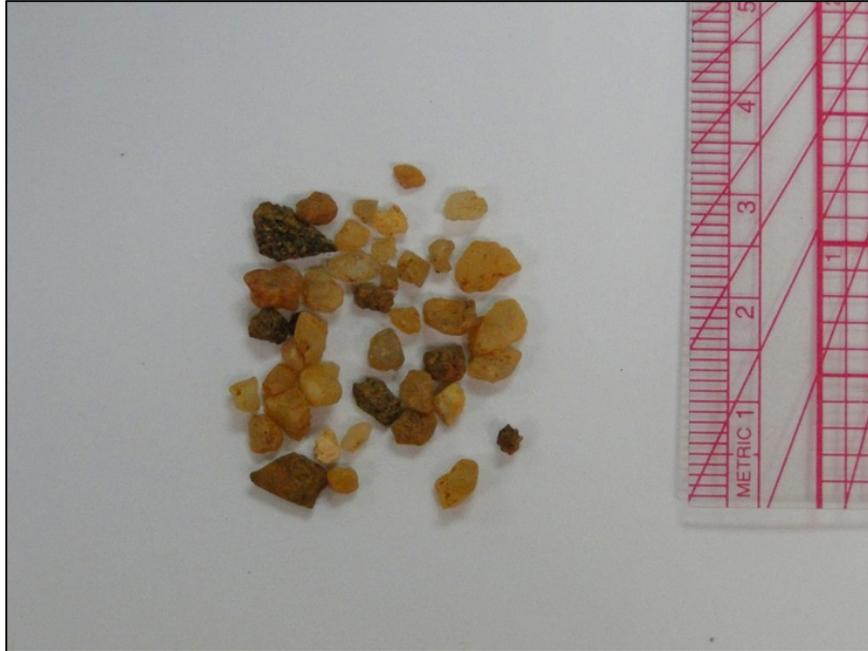
**Figure 21. Type-2 gravels have distinctly different physical properties than Type-1 gravels. This sample of the 2-4 mm fraction of a Type-2 gravel shows the abundance of quartz grains and Fe-oxide fragments.**
