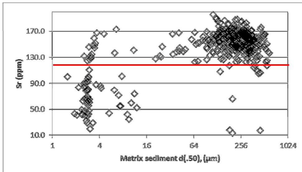
**Figure 11.** A comparison of grain size analysis d(.50) data versus Sr (ppm) of matrix sediments shows that the >120 Sr (ppm) population covers the full range of grain sizes present in this study. The <120 Sr (ppm) population is generally associated with clay grain sizes. However, there are sand samples present in this population with Sr (ppm) as low as 12 ppm. The red line marks 120 ppm. (n=418)
