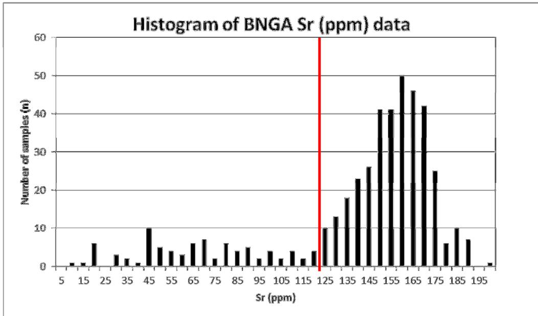
**Figure 8. The histogram of BNGA Sr (ppm) data (n=443) reveals that 81% of the samples have Sr (ppm) >120 ppm.**
