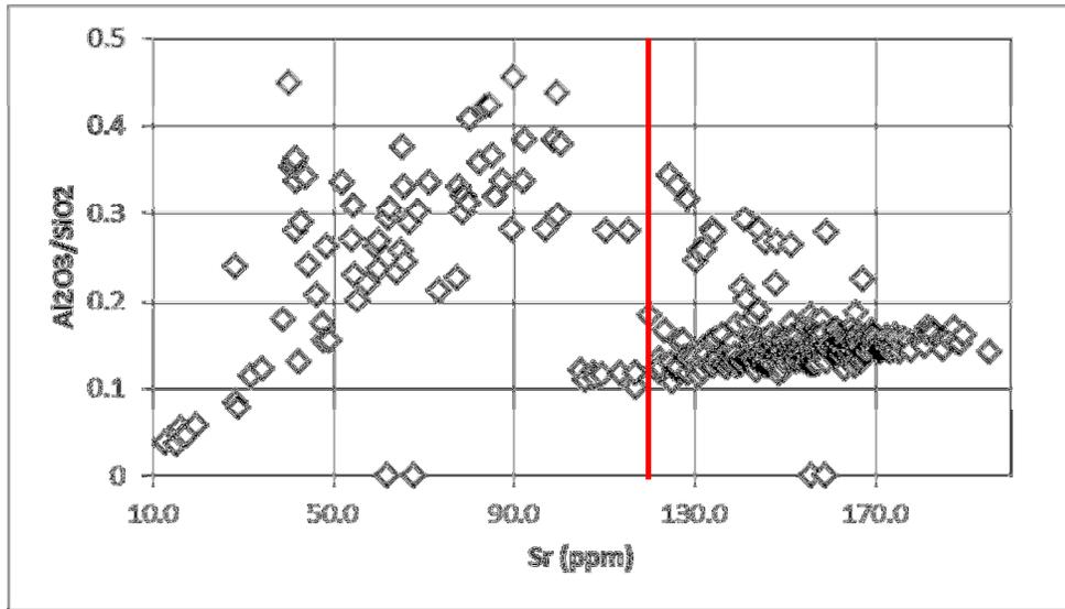
**Figure 10.** The data reveal that the >120 Sr (ppm) population is generally associated with a lower Al<sub>2</sub>O<sub>3</sub>:SiO<sub>2</sub> than the <120 Sr (ppm) population. However, used as a proxy for grain size, these data show that both the fine and coarse matrix sediments contain a wide range of Sr (ppm). The red line marks 120 ppm. (n=443)
