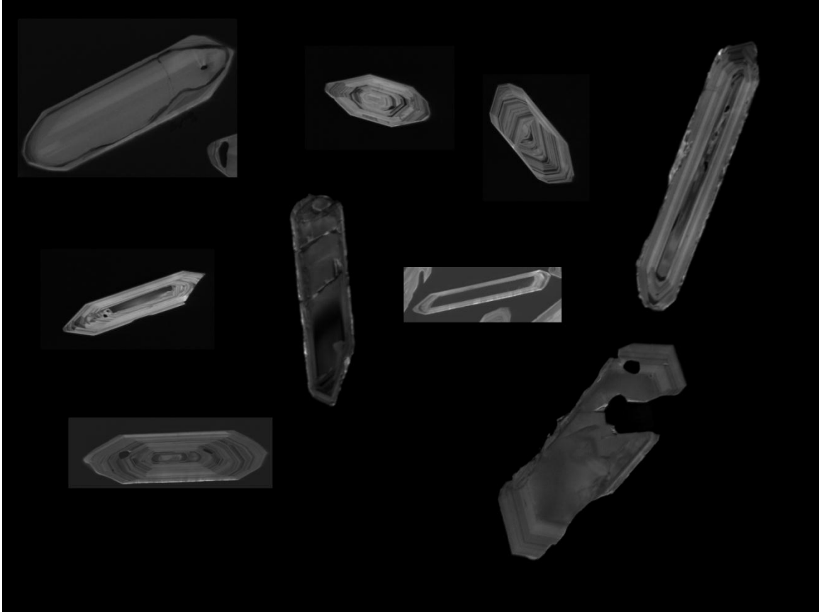
Figure 1: Cathodoluminescence images of polished zircons from this study showing typical varieties of zoning patterns. Zircons are not to scale relative to one another.
