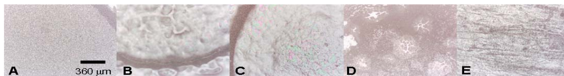
Figure 38. Progression of GOx film on the Electrode Surface Over Time. (A) Unmodified (B) 30min after GOx and Nafion are applied (C) After first calibration in RPMI (D) Film after 3 days use and storage (E) Electrode surface after lightly scrubbing with water and ethanol.
