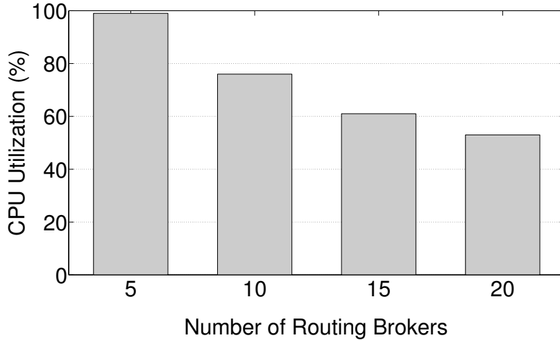
Figure 34: CPU Utilization with Load Balance in Routing Brokers
