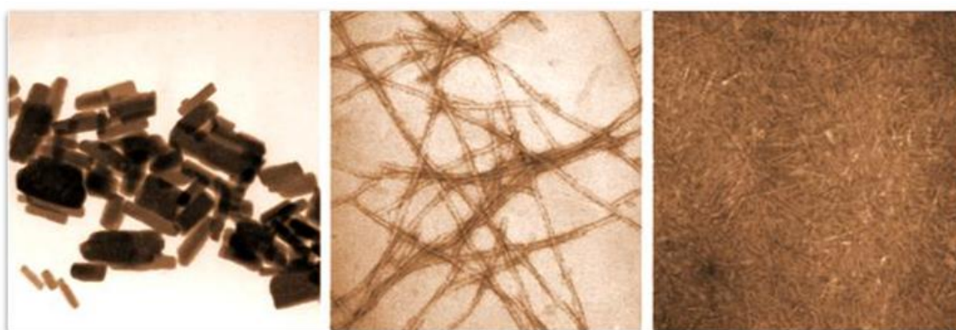
Figure 5: Transmission electron microscopy images of the nanostructures formed by the self-assembly of A 3 K (left), A 6 K (center), and A 9 K (right) peptides. [44].
