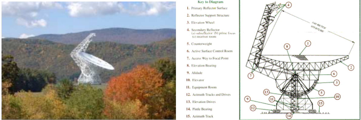
Figure 21: Left: the Robert C. Byrd Green Bank Telescope in Green Bank, WV. Right: A schematic diagram of the GBT (McKinnon, 2002)
