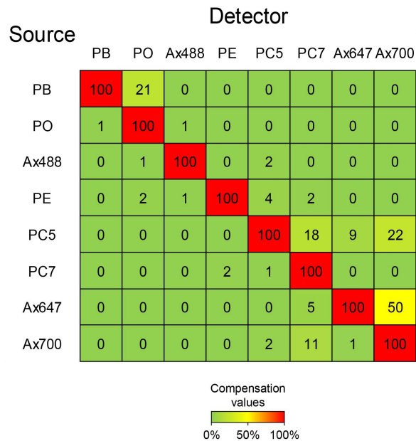
Figure B-8 Matrix depicting compensation values in an example FCB panel
