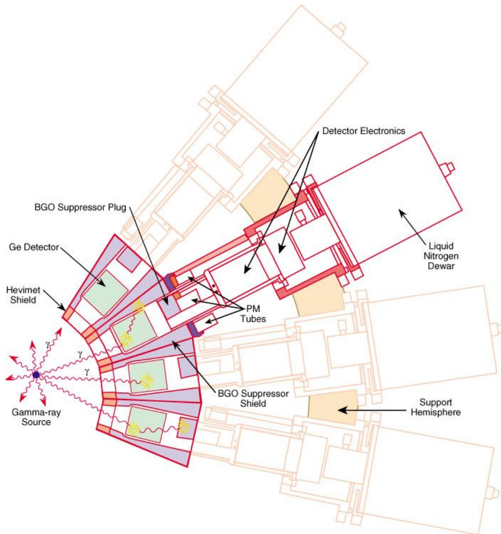
Figure 3. 1. 3 A cross section schematic of Gammasphere [5].
