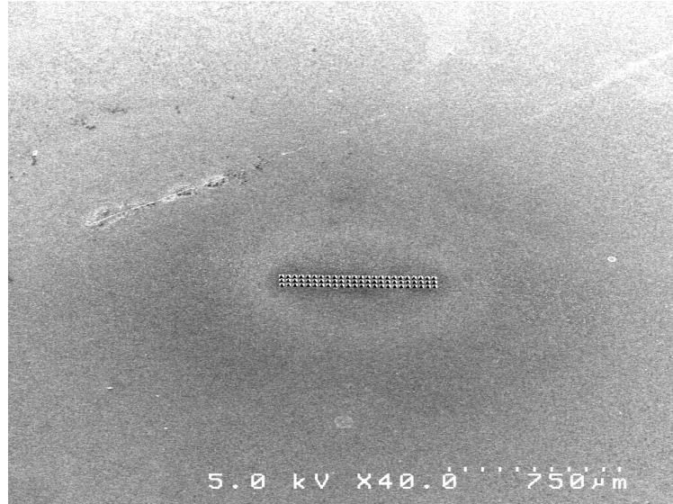
Figure 3.17: Roughly uniform distribution of back-sputtered anode material on the cathode surface following moderate current operation.
