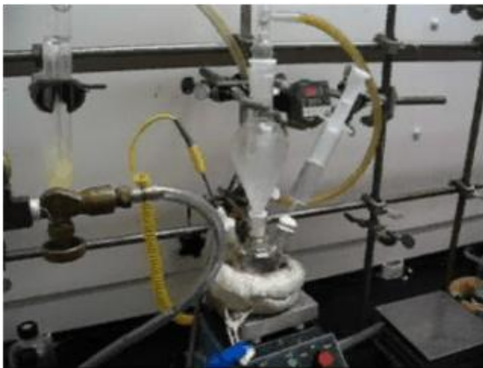
Figure 2.1: Photograph of the nanocrystals synthesis setup.
