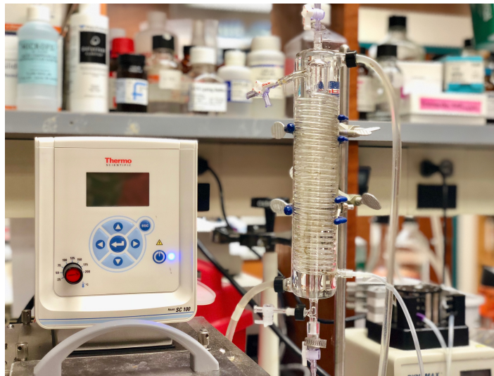
Figure 4.1 Langendorff perfusion system. An in vitro technique that allows for retrograde perfusion of the rodent heart via the cannulated aorta.
