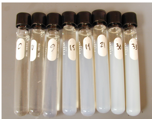
Figure 4: Calibration tubes irradiated to different doses.
