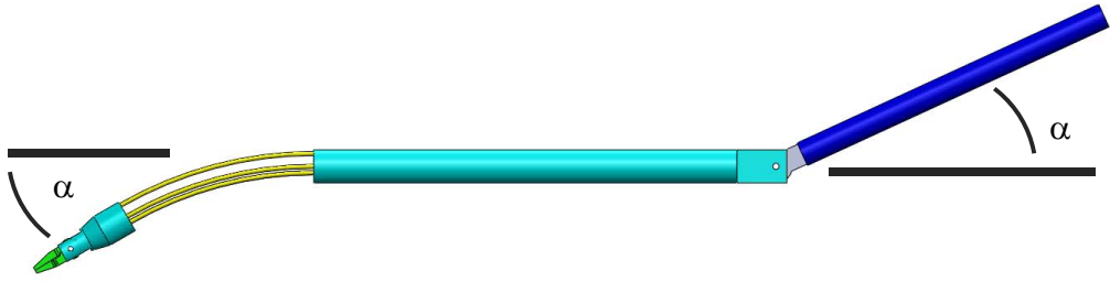
Figure 5.2: Basic conceptual layout of the continuum structure (left) and control handle (right). A mechanism is assumed to deflect the continuum structure based on the displaced angle of the control handle.
