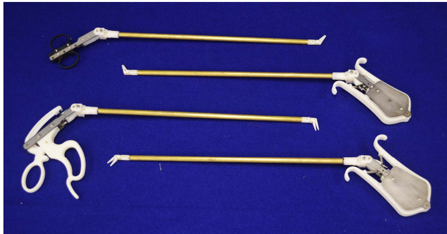
Figure 3.15: Pictured are the tools constructed for the user study. The tools are described from top to bottom. Hemostat tool (A) : Parallel mapped with a hemostat type interface. This test tool is similar to the EasyGrasp and DragonFlex research tools. Prototype tool B : Parallel mapped with a user handle intended to co-locate the proximal wrist control joint and the virtual reference frame of the hand (the point of grasp of the first finger and thumb). Pistol grip tool (C) : Anti-parallel mapped tool with pistol grip type interface. This test tool is similar to the commercial Real-Hand and CambridgeEndo tools. Prototype tool D : Anti-parallel mapped version of tool B.
