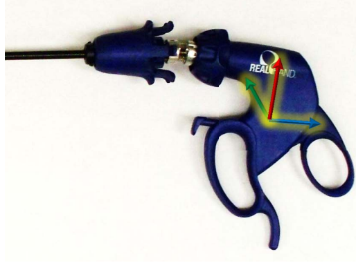
Figure 3.11: The designated location of the RealHand's origin. This location is shown as representative of the origin location for devices using a pistol style grip.
