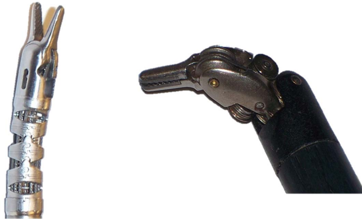
Figure 4.4: Types of Wrists: Grasper plus wrist (left), finger-wrist (right). The grasper mechanism of the grasper plus wrist design is mechanically independent of the wrist mechanism. The cables which articulate the wrist are independent of those which operate the grasp. In the finger-wrist design the coordinated movements of the fingers (both up, both down) provide a wrist DOF. The cables which open and close the grasp also operate a wrist DOF. (Intuitive Surgical EndoWrists used as examples)
