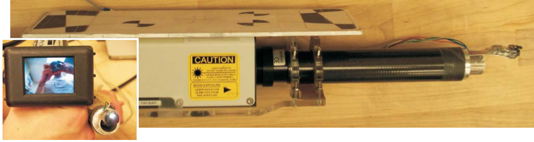
Figure 2.19: First prototype of a laparoscopic tube attached to the Conoprobe. A small CCD camera is attached to the tip of the tube, enabling the physician to view the position of the laser measurement spot on a hand-held display screen. The inset image in the lower left shows the display screen and the tip of the tube seen end-on. This first prototype illustrates the basic concept but is not yet airtight.
