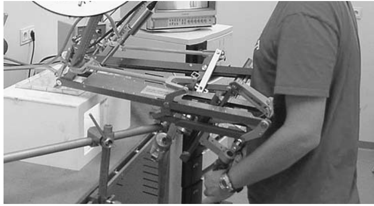
Figure 3.4: Manually actuated, dexterous surgical system based on pantograph mechanism [46].
