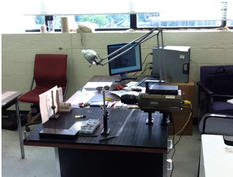
Figure 5.5: The experimental setup for high-speed imaging of the wing motion.
