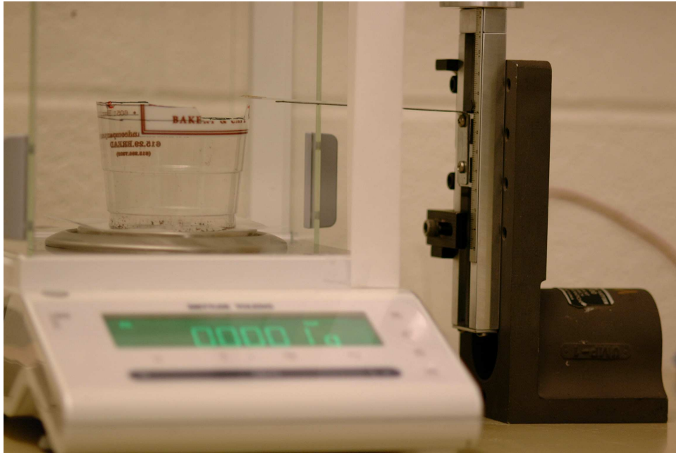
Figure 5.3: The experimental setup for stiffness measurement.
