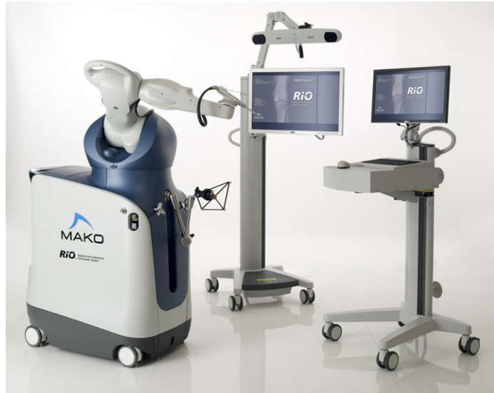
Figure 1.17: RIO Robotic Arm Interactive System for orthopedic surgery (makosurgical.com).
