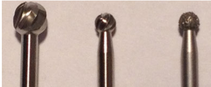
Figure 2.7: Photograph of surgical cutting burrs used in experiments; from left to right: 5 mm fluted, 3 mm fluted, and 3 mm diamond coated burr
