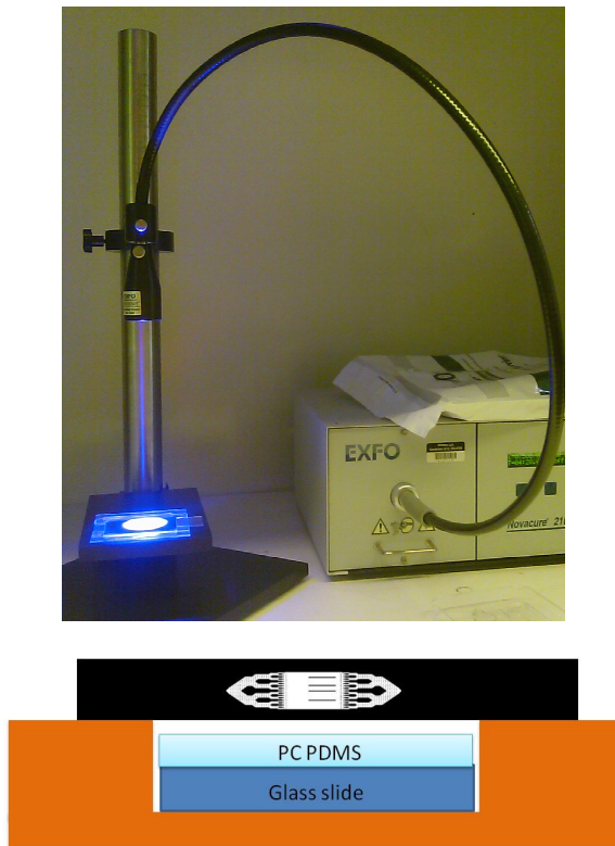
Figure 34. PC PDMS photoinitiation achieved using UV light. The top figure shows the collimating adapter used to direct light to the substrate. The bottom figure shows the typical setup for laying the mask over the PC PDMS by attaching it on both sides to two thick (1.5 mm) glass slides. The glass slide the PC PDMS was on was only 1.0 mm. The thick glass slides were bound via epoxy to allow for easy transfer of the PC PDMS into the appropriate position for UV exposure.
